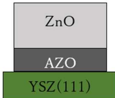
Figure 2: Layout of AZO-ZnO heterostructure deposited on a YSZ substrate
