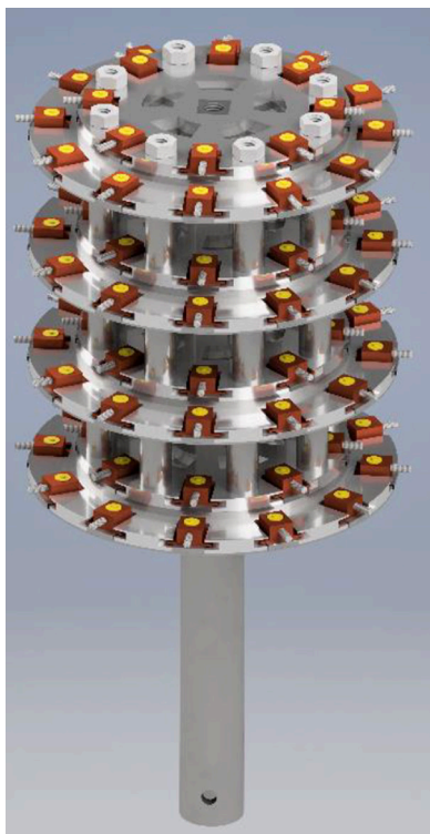
Figure 2: Storage sample garage.
