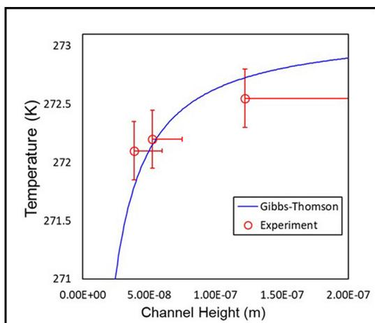
Figure 4: Melting temperatures of ice in nanochannels with different channel heights compared to the Gibbs-Thomson prediction. Values agree with those predicted by the Gibbs-Thomson relation.
