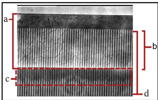
Figure 3: Image obtained from freezing experiment. (a) Microchannel containing bulk ice, identified by the grain boundaries present in image. (b) 500  $\mu\text{m}$  channel overlap. (c) Liquid water in nanochannels (darker region) coexisting with ice (brighter region) at subfreezing temperature. (d) Nanochannel array.
