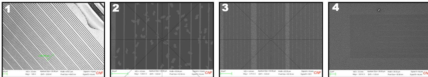
Figure 1: SEM image of various width patterns (largest 1000 nm) of Zn-oxide NP resists. Figure 2: SEM image of a 1000 nm-width pattern from the Zn-oxide NP resist. Figure 3: SEM image of a 500 nm-width pattern (center) from the Zr-oxide NP resist. Figure 4: SEM image of a pattern exposed region from the CARs.
