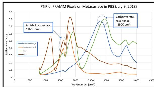
Figure 1: Reflectance spectra of FRAMM and nanoantenna pixels in PBS, tuned to match amide I and carbohydrate resonances.
