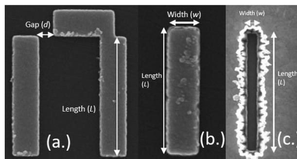
Figure 2: SEM images (taken at 20.00 kV) of (a) FRAMM (pi), (b) nanoantenna, and (c) nanoslit structures.
