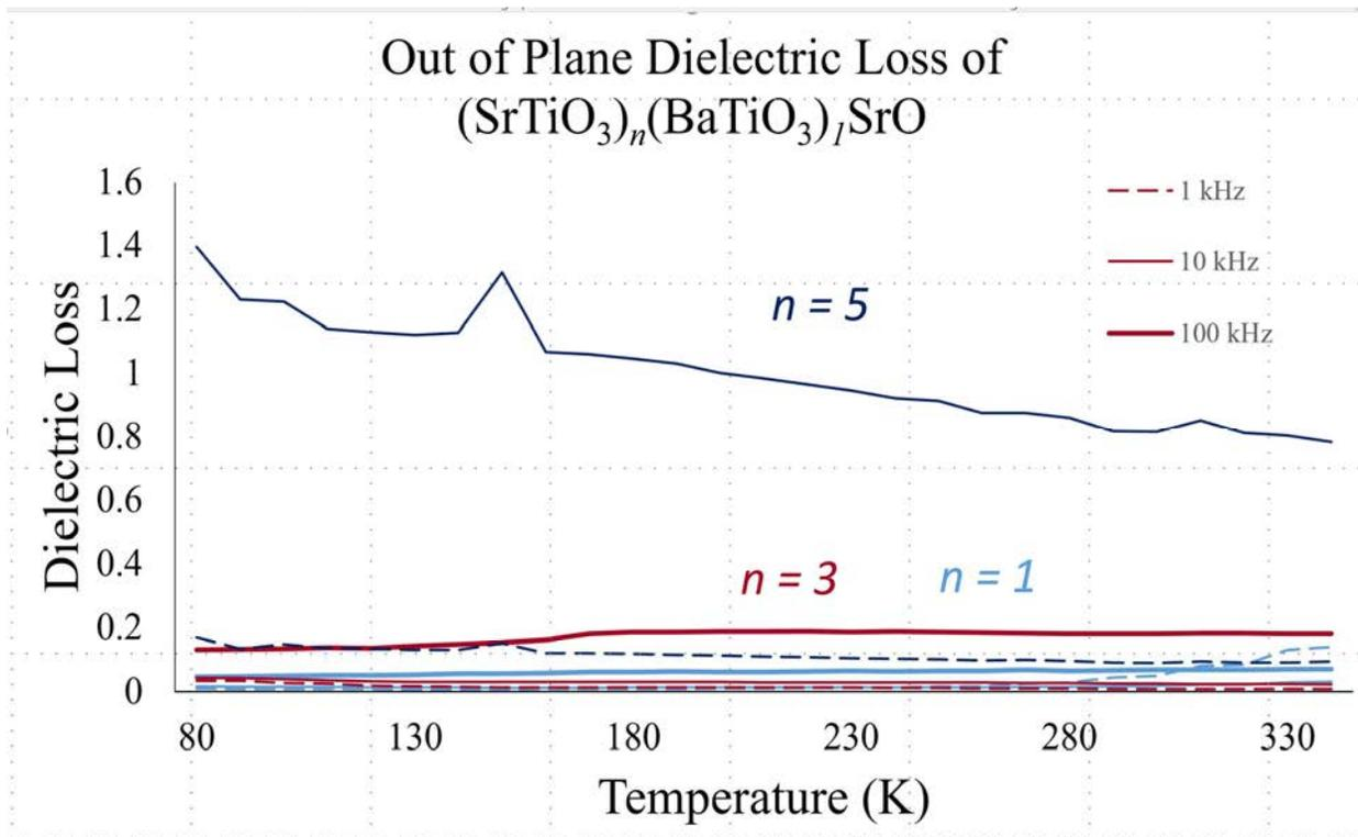
Figure 11: Comparing the top graph and the bottom graph, it is very clear that out-of-plane overall has greater dielectric loss, especially for  $n=5$ .
