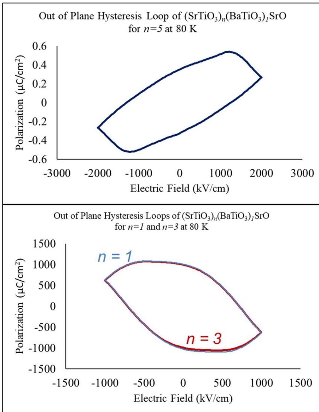
Figure 5: The top graph for the sample  $n=5$ , while indicating reasonable looking polarization values, indicates leakage from the shape. This leakage is made much more clear in the  $n=1$  and  $n=3$  samples in the bottom graph, which shows unreasonable polarization measurements.
