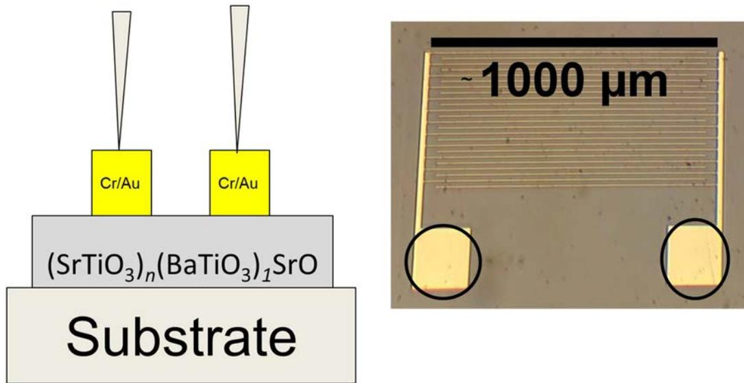
Figure 8: On the left, the structure of the in-plane sample can be seen. The  $(\text{SrTiO}_3)_n(\text{BaTiO}_3)_1\text{SrO}$  thin film (with thickness of 100nm) was deposited on the  $\text{DyScO}_3$  substrate. The Cr/Au electrodes were patterned as interdigitated electrodes, and the probe tips contacted these electrodes. On the right, the interdigitated electrodes used is shown, with contact points circled.
