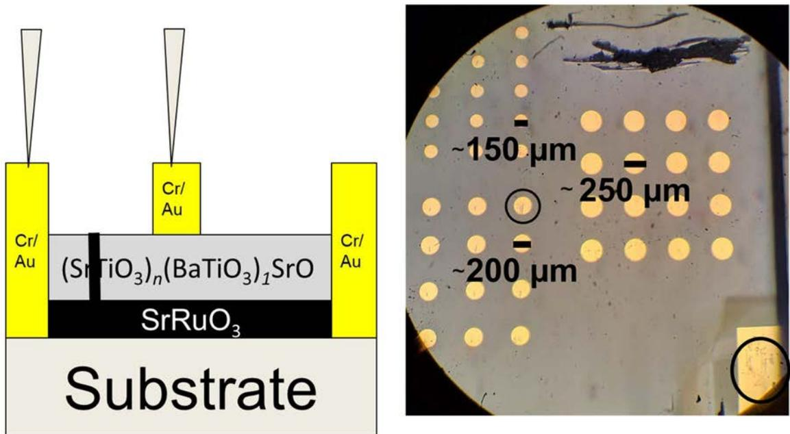
Figure 9: On the left, the structure of the out-of-plane is shown, which is similar to in-plane except for the deposited 15 nm layer of  $\text{SrRuO}_3$ . To contact the  $\text{SrRuO}_3$  layer, the bottom electrode, a probe tip contacted the corner Cr/Au. The other tip was placed on a circular pad as the top electrode. The right shows the circular pads, their sizes, and the corner pad. Contact points are circled.
