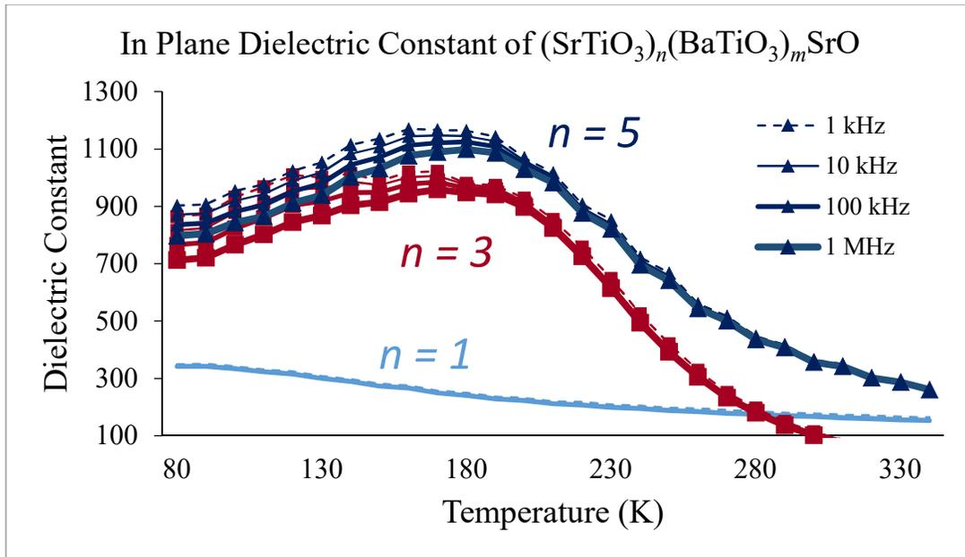
Figure 3: For  $n=1$ , there is no peak that would be indicative of a ferroelectric transition. In contrast, for  $n=3$  and for  $n=5$ , there are peaks indicating ferroelectric properties.
