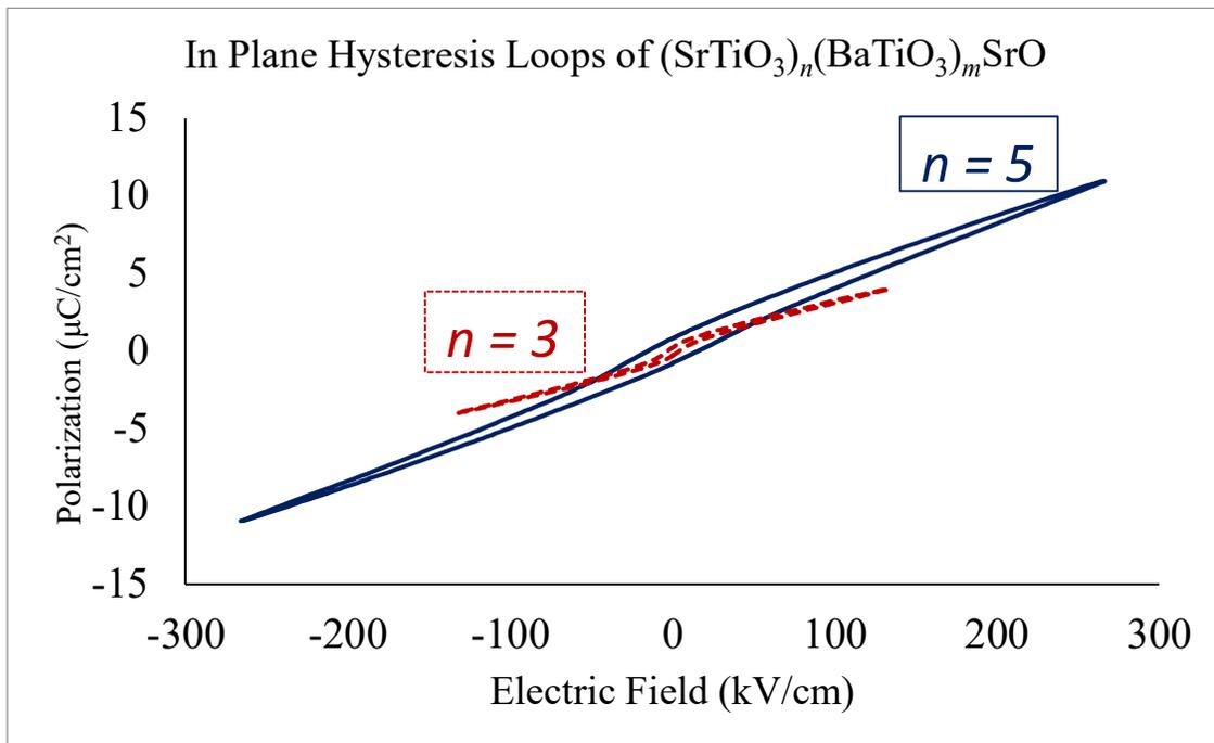
Figure 4: The shapes of the hysteresis loops indicate presence of ferroelectric properties (though probably not that strong).
