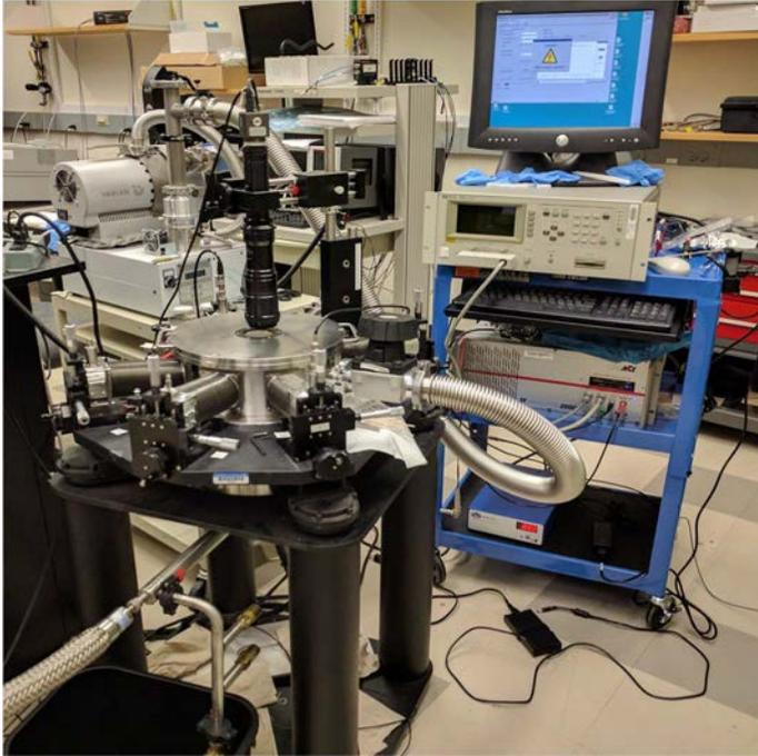
*Figure 7: The cryoprobe, on the left, was used to contact the electrodes and allowed for measuring at low temperatures. The cart, to the right, has the dielectric tester at the top, and the ferroelectric tester on the shelf below.*
