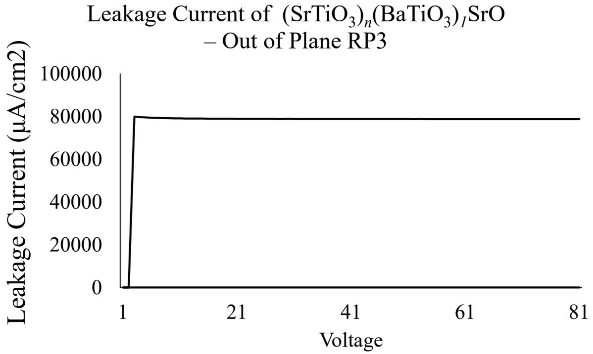
Figure 10: This measurement shows that for even voltages as low as perhaps 5V, the leakage current measured is extremely high.
