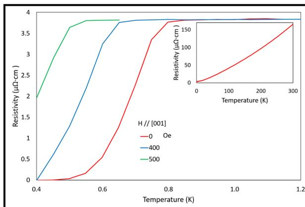
Figure 2: Resistivity as a function of temperature ( $< 1.2$  K) under various magnetic fields applied parallel to the  $c$ -axis of the film. Inset shows resistivity as a function of temperature up to room temperature.
