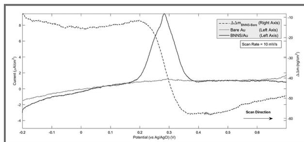
Figure 3: Oxidation sweeps (solid lines) for bare Au and BNNS/Au and difference in adsorbed mass,  $\Delta\Delta m_{\text{BNNS-Bare}}$  (right axis).
