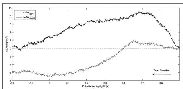
Figure 2: Mass of adsorbed oxygen with respect to potential for bare Au and BNNS/Au.
