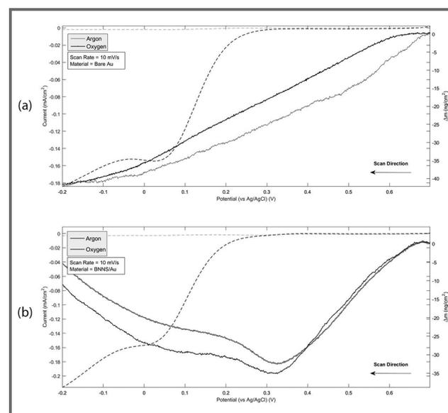
Figure 1: Reduction sweeps (left axis) and  $\Delta m$  (right axis) for bare Au electrode (a) and BNNS/Au (b).
