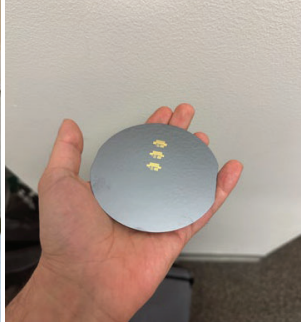
Figure 2b Wafer after Lift-off with designed metallic patterns.
