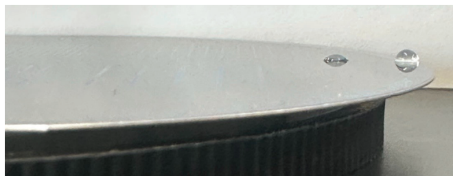
Figure 2: Water droplets on silicon wafer demonstrating biphilic pattern formation.
