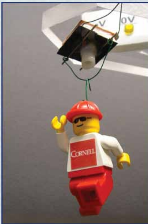
Figure 1: Paul Steen and Michael Vogel’s surface tension-based adhesive device with a lego man payload. The researchers demonstrate a larger version of their switchable adhesive device in a video, http://www.news.cornell.edu/stories/Feb10/adhesive.html
