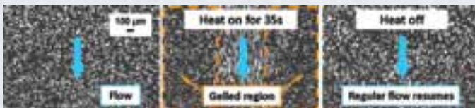
Figure 2: Dynamic channel creation and reconfiguration. A narrow straight channel created within a larger microfluidic chamber by selective heating along the sides. The original flow field was obtained on turning the heat off.
