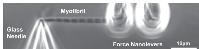
Figure 1: Example myofibril held between a glass needle and force nanolevers imaged under phase contrast.
