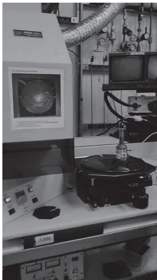
Figure 1: Cathodoluminescent lamp and temporary support fixture positioned over the ABM Mask Aligner wafer stage for the initial exposure experiment.
