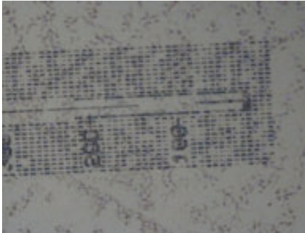
Figure 2: Snapshot of sample with the MIBK and IPA mixture with HSQ that is damaged
