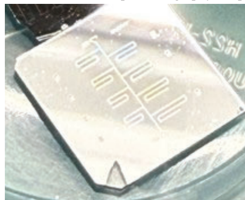
Figure 1: Fabricated Al-on-sapphire resonator chip showing patterned resonator structures on the top surface.
