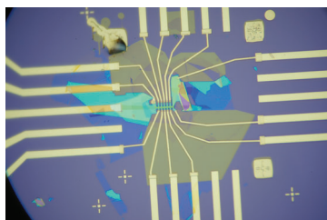
A rhombohedral-stacked multilayer graphene heterostructure which has been etched into a Hall bar geometry using nanofabrication facilities.
