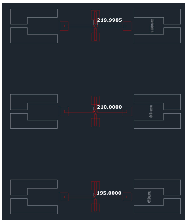
Fig. 1: STM_v2 mask design showing 3 \mu m alignment markers.
