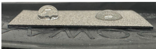
Figure 3: Water droplets on titanium porous transport layer with a simplified biphilic pattern.
