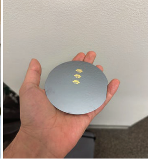
Figure 2b Wafer after Lift-off with designed metallic patterns.
