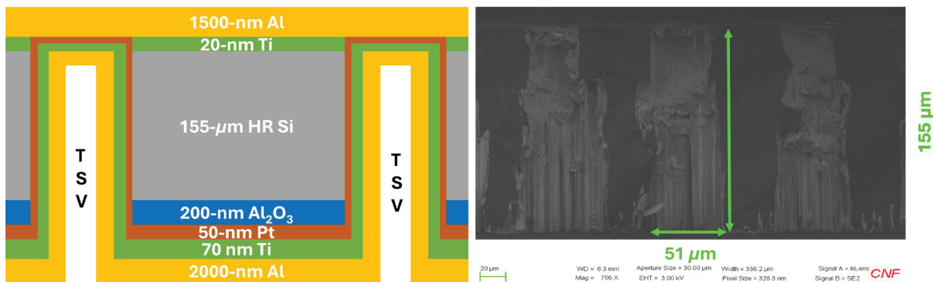
Fig. 2. Cross-section (a) schematic and (b) SEM image of a metallized through-Si via (TSV).
