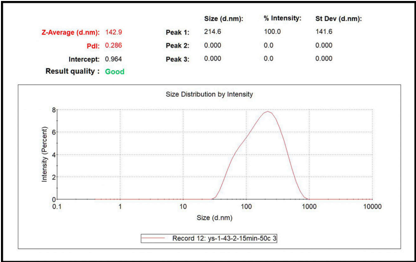
Figure 3: DLS of emulsion made by CoFe 2 O 4 NPs and preceramic precursors at 50°C.
