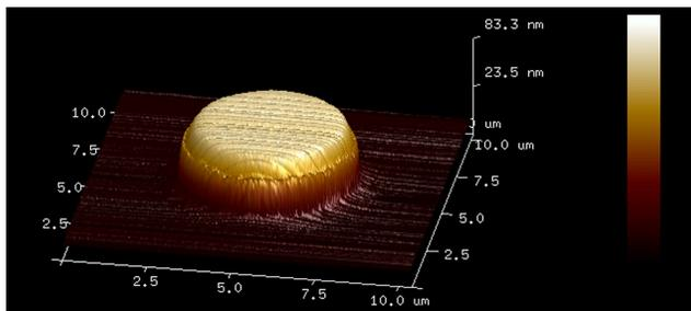
Figure 2: 3D AFM image of 5  $\mu\text{m}$  diameter circular pillar after argon ion milling, showing smooth edges and absence of “rabbit ears” characteristic of lift-off process using deposition via sputtering.
