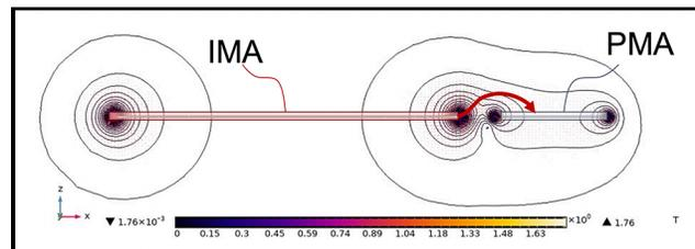
Figure 4: Magnetic simulation of IMA and PMA magnets spaced 1.5  $\mu\text{m}$  away from each other. The contour lines show the change in magnitude of the magnetic flux density. The red arrow emphasizes the direction of magnetic flux closure from the IMA to the PMA magnet.
