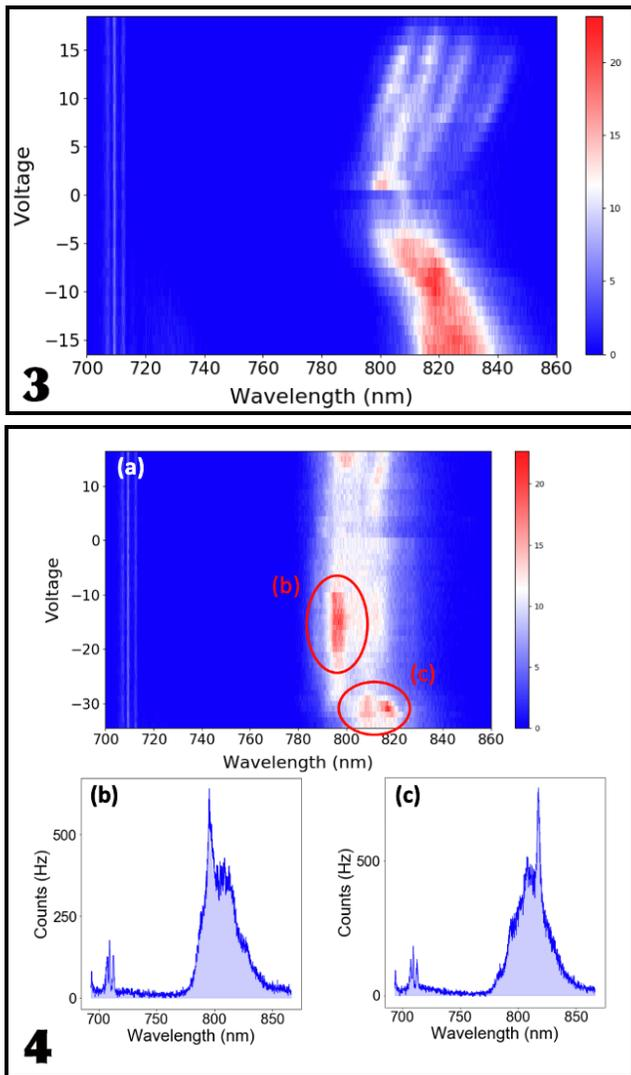
Figure 3, top: Photoluminescence modulated by  $V_{gb}$ .  $V_{tg}$  is adjacent to 2L-WSe<sub>2</sub>, and it directly pumps charge carriers into 2L-WSe. We can see a clear doping effect. Figure 4, bottom: (a) Photoluminescence modulated by  $V_{tg}$ .  $V_{gb}$  is adjacent to BTO, and it switches the polarization in BTO. (b) and (c) show the change in population proportion of  $\Lambda - K$  and  $\Lambda - \Gamma$  indirect excitons under the polarization switching in BTO.
