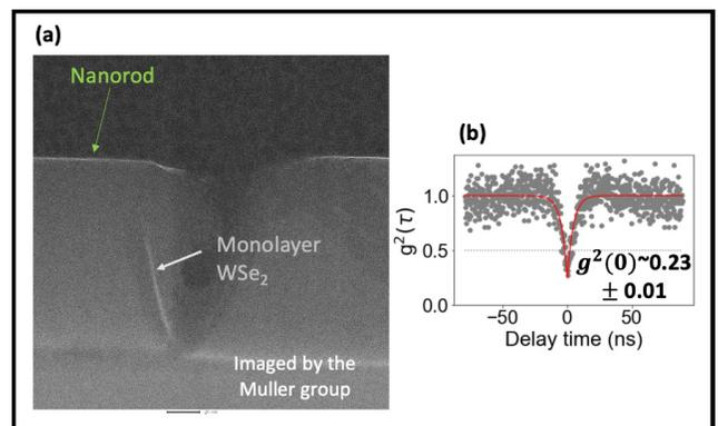
Figure 2: (a) TEM image of a nanogap site with the sharply folded monolayer  $\text{WSe}_2$ . (b) Time correlation measurement of a quantum emitter created at the sharp fold in (a).  $g^2(0)$  is 0.23, which shows a single photon nature of the emitter.
