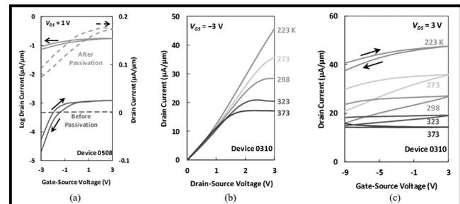
Figure 2: (a) Drain current under different gate-source voltages in log and linear scale,  $V_{DS} = 1$  V, (b) output curves ( $V_{GS} = -3$  V) and (c) transfer curves ( $V_{DS} = 3$  V) of device 0310 under different temperatures (223, 273, 298, 323, 373 K).
