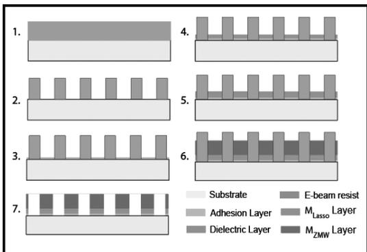
Figure 1: Schematic representation of ZMW fabrication process: 1. Spincoat negative e-beam resist and bake. 2. Expose using e-beam lithography and develop resist. 3. E-beam evaporation of an adhesion layer on the fused silica substrate, followed by deposition of Pt layer (electrode), alumina (dielectric layer), and 100 nm aluminum (cladding layer of ZMWs). 4. Lift-of-resist using 1165 stripper.
