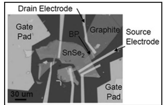
Figure 1: Optical image of the representative BP/SnSe<sub>2</sub> TFET.
