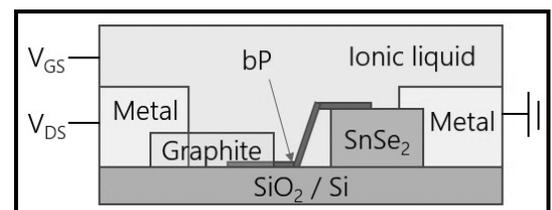
Figure 2: Cross-sectional schematic image of the device.
