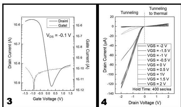
Figure 3, left: Current as a function of gate voltage at V<sub>DS</sub> = -0.1 V at room temperature in N<sub>2</sub>. The black line indicates drain current and the red line indicates gate leakage current. Figure 4, right: Drain current as a function of drain voltage with different gate voltages.
