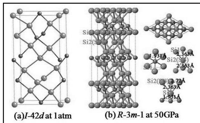
Figure 1: Predicted I-42d, and R-3m-1 structures for  $\text{Si}_3\text{C}$  at 1 atm, and 50 GPa, respectively. Orange, large balls are Si; grey, small balls carbon. The right panel of (b) presents the top view of the R-3m-1 structure and Si-or C-centered octahedra within the structure. See full color version on pages xxviii-xxix.
