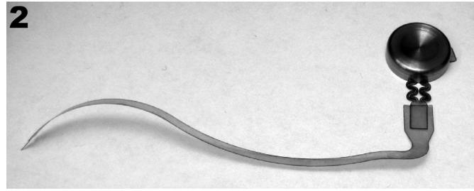
Figure 2, above right: A picture of a VersaLaser-cut mechanical mockup of an indwelling brain electrode system including a titanium hermetic enclosure.
