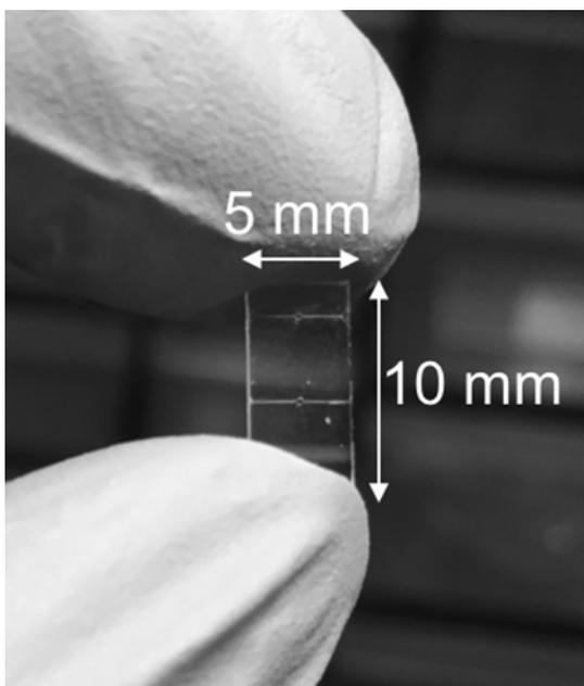
Figure 3: Snapshots of the completed side-coupled microfluidic device.
