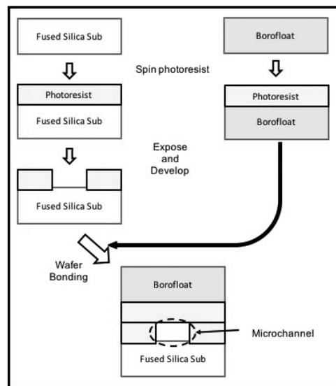
Figure 1: Process flow of fabricating side-coupled microfluidic devices.
