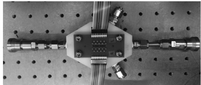
Figure 3: Package with external electrical connections.
