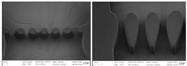
Figure 1: Scanning electron microscopy (SEM) images of circular (left) and hydrofoil (right) pillars.
