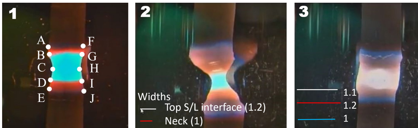
Figure 1, left: Landmarked image of a healthy molten zone marking the edge of the top rod (A,F), top of the molten zone (B,G), “neck” of the molten zone (C,H), bottom of the molten zone (D,I), and edge of the bottom rod (E,J). Figure 2, middle: Thinning molten zone due to user error. Respective widths of various parts of the molten zone characterize it as unhealthy. Figure 3, right: Convex molten zone characterized by the neck of the molten zone being the widest point.
