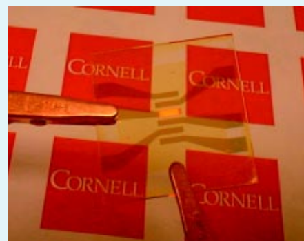
Figure 3: A sandwich structure device in operation with air stable electrodes.
