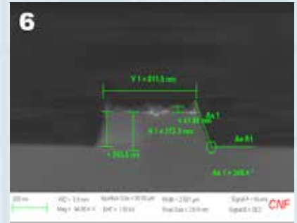
Figure 6: Silicon nitride etch using CH_2F_2/He in Oxford 100 ICP. The CH_2F_2/He chemistry is highly polymerizing and therefore highly selective with respect to imprint and conventional photoresists.
