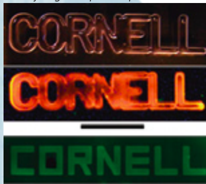
To demonstrate that DNA hydrogels will hold their shape for such applications as tissue engineering, Cornell researchers molded samples to spell out "CORNELL." The sample at the top, about three centimeters long, is stained with a dye that fluoresces red under ultraviolet light (center). The sample at the bottom, about 3,500 microns (millionths of a meter) long, was created in a mold etched into a silicon chip at the Cornell NanoScale Facility and stained with a green fluorescent dye.
