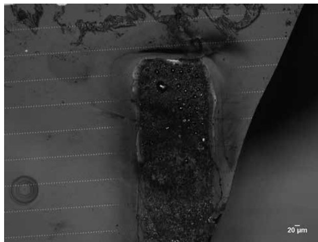
Figure 1: Bright field micrograph of GaN on sapphire sample with gold dots annealed with a single laser scan.
