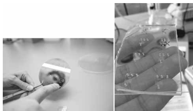
Figure 2: Left: SU-8 wafer with patterned structures. Right: A series of eight PDMS microfluidic devices.
