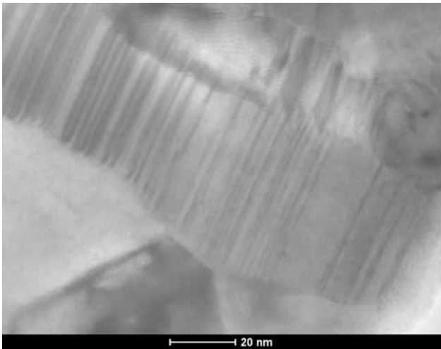
Figure 2: A magnified TEM image of one of the small grains near the surface of the Cu film visible in Figure 1. This image shows coherent twin boundaries (alternating dark and light striped regions) that occur with an average spacing of about 1 nm or less.
