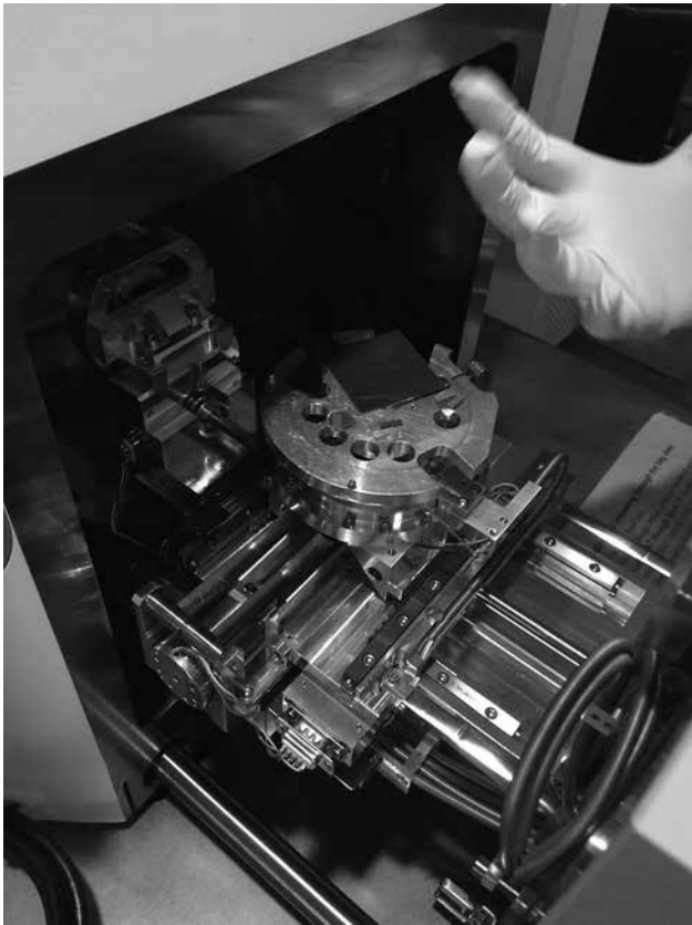
Figure 1: Metals being loaded into SEM after growth for analysis.
