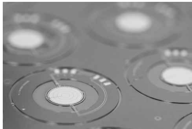
Figure 1: MEMS three-dimensional micro-mirror post release.
