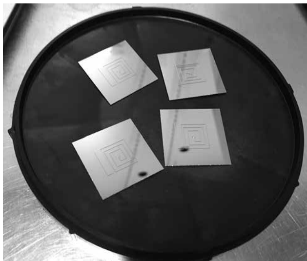
Figure 2: Completed masters for hot embossing.
