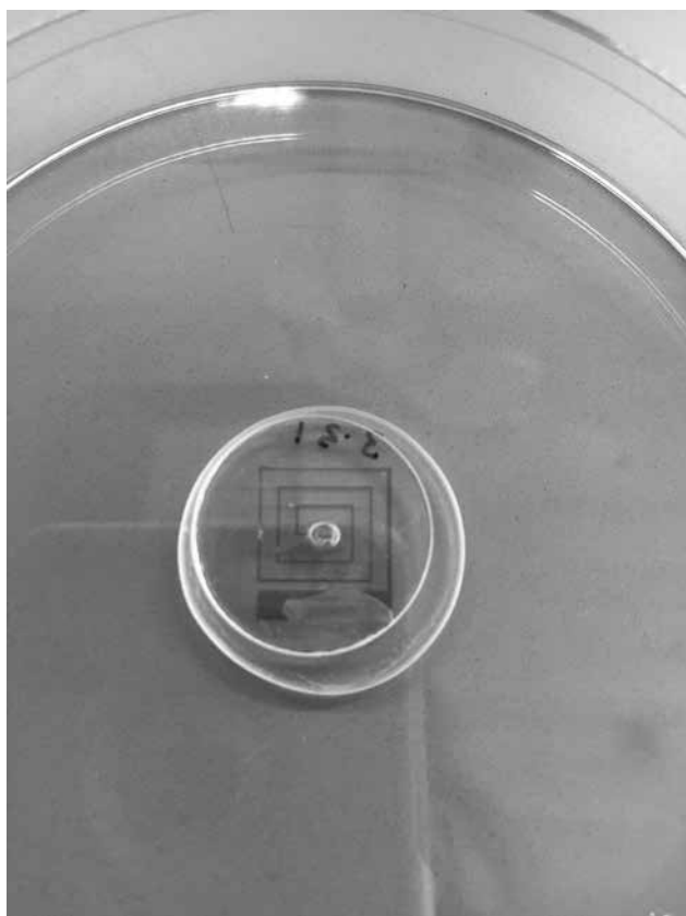
Figure 3: Completed microfluidic chip with blue dye shown for visualization of channels.
