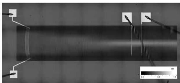
Figure 3: Another device. A curved IDT, left, creates a SAW that propagates right to an invisible piece of graphene placed across two electrodes. The SAW is concentrated at the graphene location.
